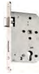
Mortise Fire Rated Lock Body Backset: 55mm, C/C: 72mm Finish- SSS
