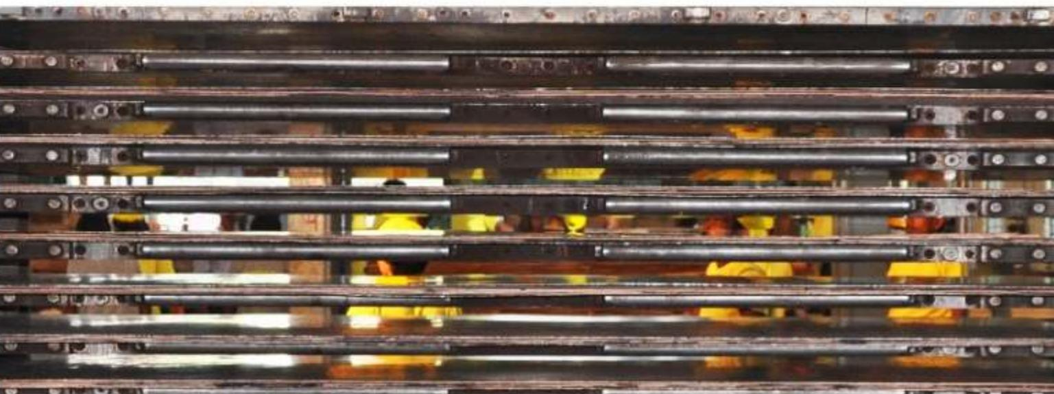
Star ply is manufactured on the philosophy of high pressurized glue line. HPGL technology helps to infuse the resin deeper in core as well as in panel. When assembled panel are pressed in hydraulic press then resin reaches uniformly to all layers (core and panels) of plywood and thus the bonding we get through this process is higher than the plywood manufactured without this process.
